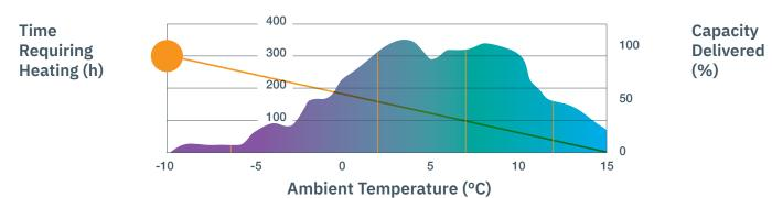
The calculation for heating is very similar to cooling. A design condition is selected at -10°C as the 100% value. Four points are then selected at -7°C, +2°C, +7°C and +12°C for part load conditions. The COPs are used to calculate energy consumed. These figures are totalled to give an SCOP when the unit is operating in heating mode. **Example:**
